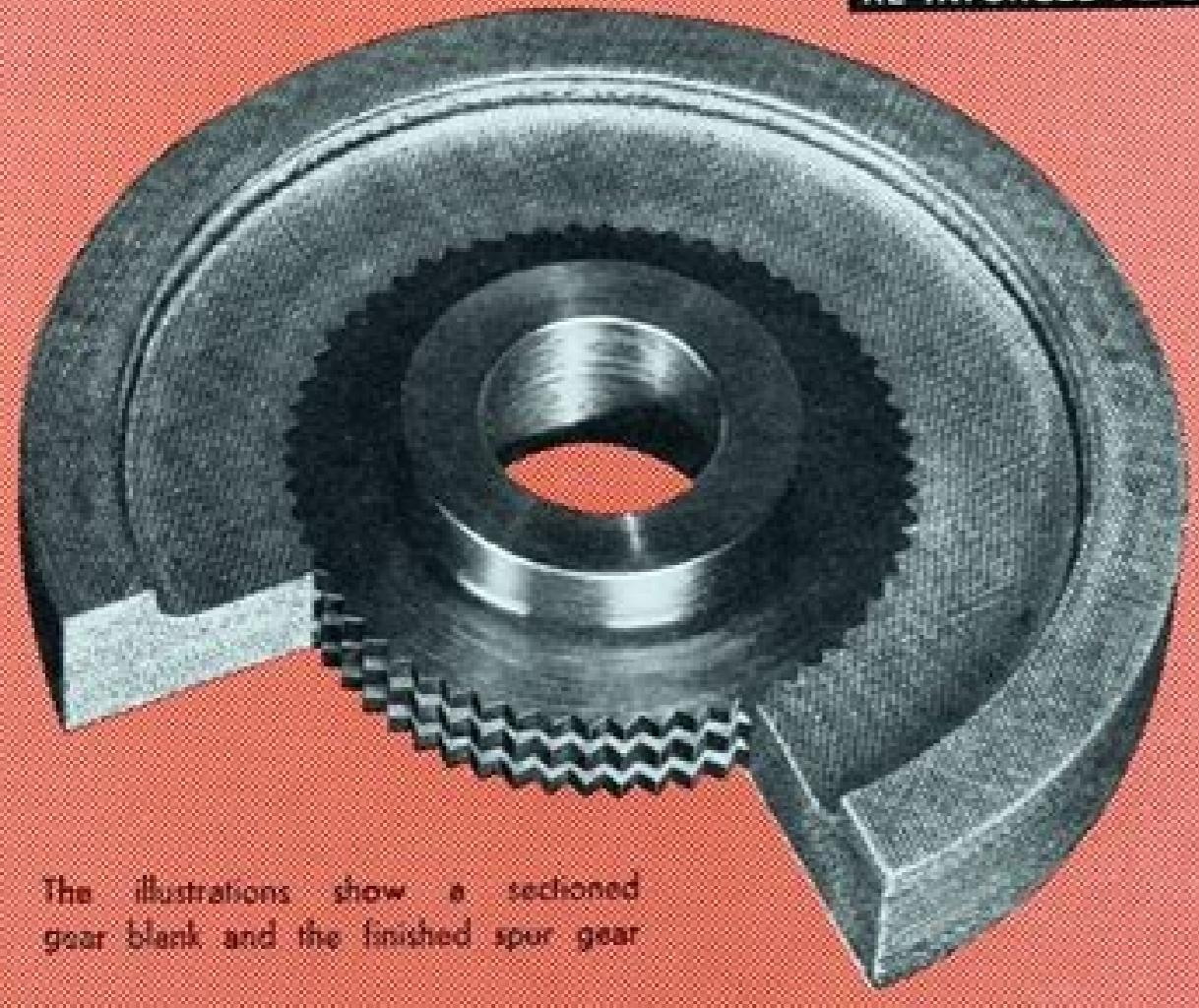
The illustrations show a sectioned gear blank and the finished spur gear
